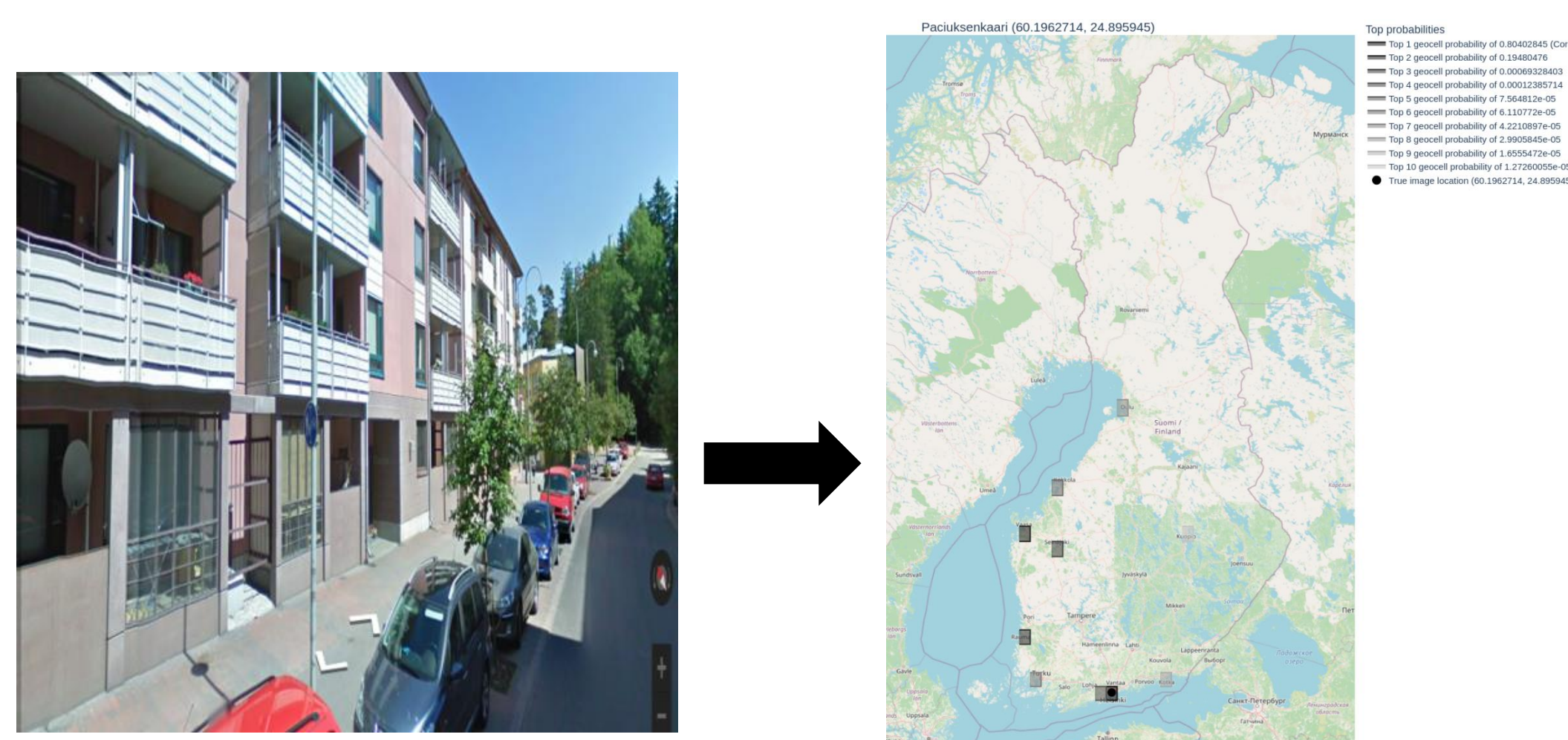
Figure 2: Trained model predicting geolocation for a sample outdoor image. Black dot indicates the true location, geocells from dark to light indicate probabilities that the image was taken there.
